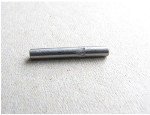
Axle “knurled” for gear
